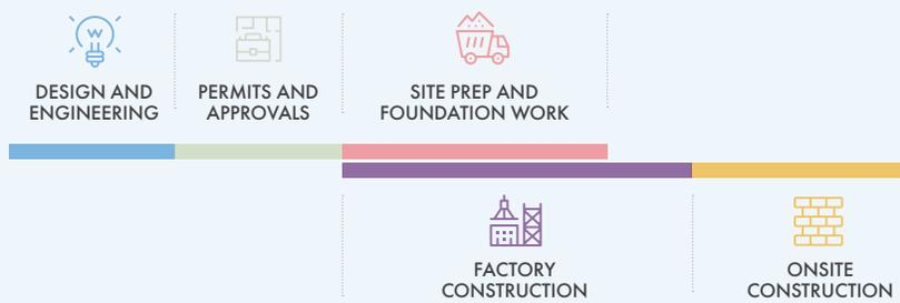
Using off-site construction to develop multifamily housing follows a unique timeline that can offer time-related cost savings.
